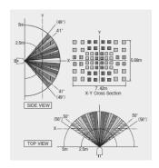
The movement detection area for small movements at a mounting height of 2.8m is about 4x6m, for large movements it is about 6x8m. Max. height for small movement detection is 3,5m.
