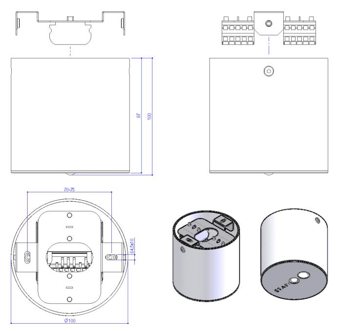
Cable entry can be done from above. Although enough connections are provided for through wiring, it is advised to use a separate connection box in case of throughwiring (especially if 2,5mm² is used) or where side entry is the only option. In these cases use a rigid surface mount connection box or cable trunk system to mount the C1C30-B to.
